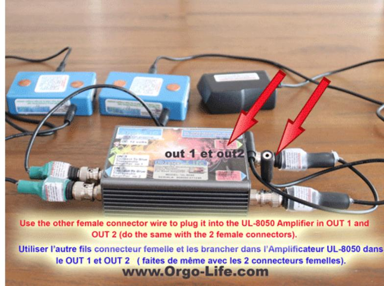
Use the other female connector wire to plug it into the UL-8050 Amplifier in OUT 1 and OUT 2 (do the same with the 2 female connectors).
