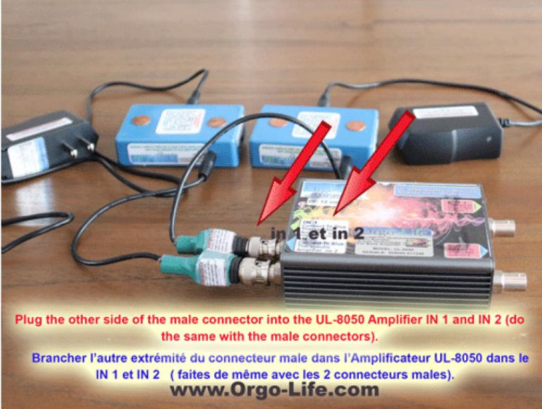
Plug the other side of the male connector into the UL-8050 Amplifier IN 1 and IN 2 (do the same with the male connectors).
