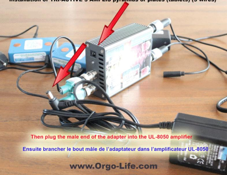
Then plug the male end of the adapter into the UL-8050 amplifier
